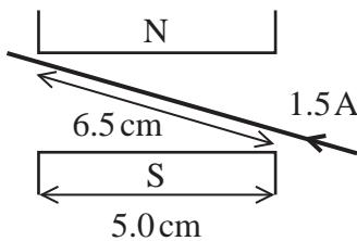
Which of the following gives the magnitude of the force on the wire, in newton, and its direction?
