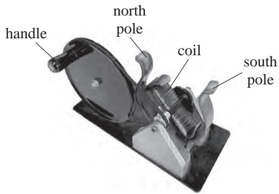
The handle is used to rotate the coil between the magnetic poles.
