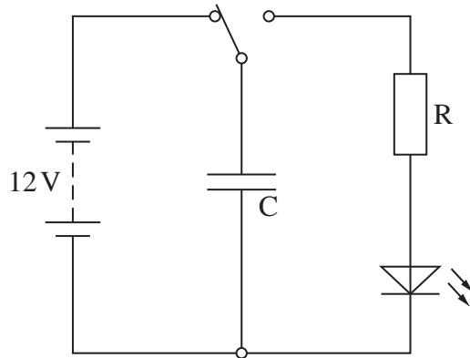
The student uses a light emitting diode (LED) and a resistor R. The LED stops emitting light when the potential difference across it falls to 1.4 V. The student assumes the LED has a constant resistance of  $340\ \Omega$ .
