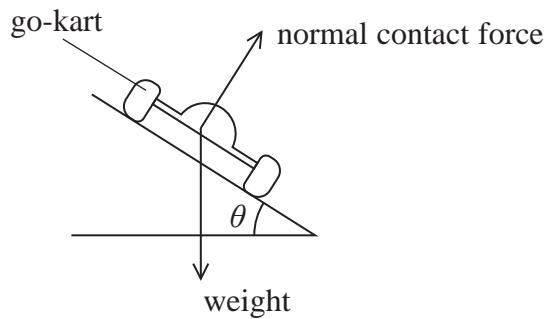
At a particular speed  $v$ , the go-kart can follow the track without any frictional force perpendicular to its motion. The diagram shows the forces on the go-kart as it is moving away.
