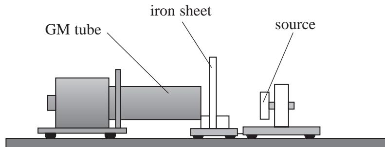
The student used five different thicknesses of iron and determined the count rate for each thickness.
