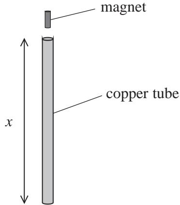
The student dropped the magnet into the copper tube and measured the time  $t$  for the magnet to reach the bottom of the tube.
