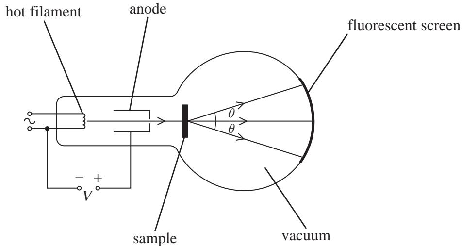
A beam of electrons is directed at a sample of crystalline material.
