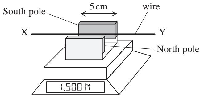
The magnetic flux density between the magnets is 0.07 T.
