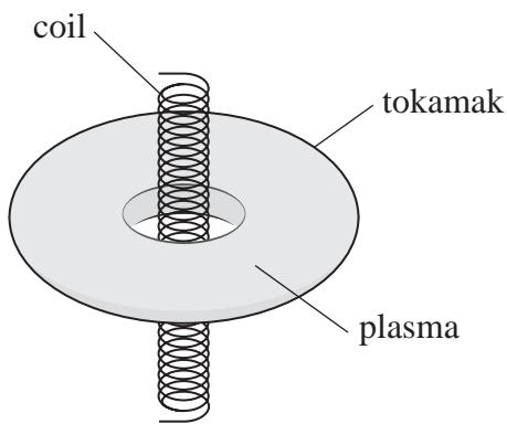
The plasma in the tokamak acts as a single conducting loop around the central coil.
