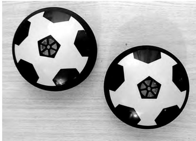
The pucks each contain a small fan, so that they glide across the table on a cushion of air. The mass of the pucks can be varied by attaching small masses.
