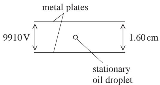
Calculate the charge on the oil droplet.
