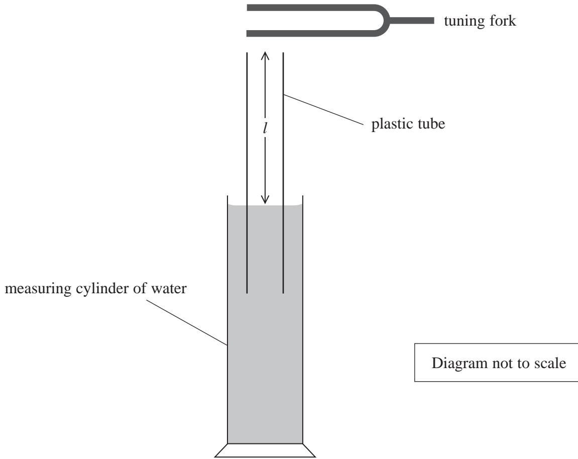
The student adjusted  $l$  until the loudest sound was heard, indicating that a standing wave had formed. He marked the water level on the plastic tube and measured  $l$ .
